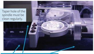
Γwo sides of water outlet must be cleaned up mmediately every day,and ensure no large amount of dust accumulation.
