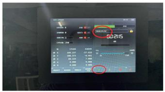
5.After the program is completed, press the "Manual" mode again, open the safety door, and then remove the workpiece to start the next molding step of denture processing.
