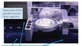
Two sides of water outlet must be cleaned up immediately every day, and ensure no large amount of dust accumulation.
